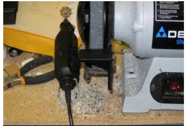
Dremel w/ cut-off Attachment Grinder -- (The width of the grinder wheel is almost perfect for grinding the shape of the light housing.)
